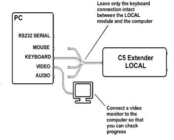
7 Switch off the computer and disconnect the KVM+A multi-cable. Leave the monitor connected and the upgrade disk in the floppy disk drive.
